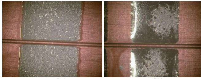
2a) 2b) Figure 2: Solder Paste a) after printing and b) after reflow
